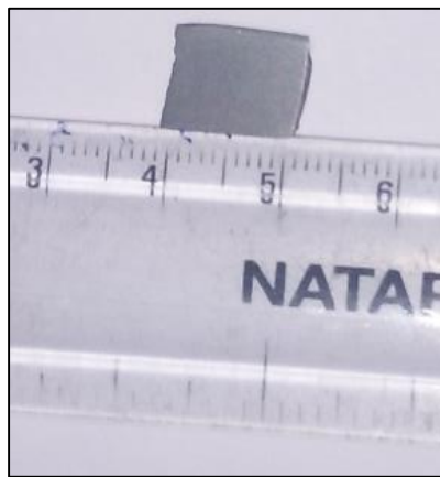
Figure 14: Prepared specimen for microstructure and hardness test
